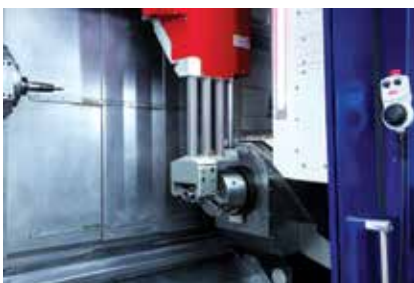
Integrated mini gantry with 2 axes
