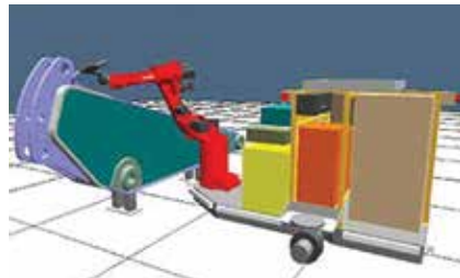
Fig.2. Schematic diagram showing autonomous robot vehicle navigated by vision system, being used for all positional MIG / MAG welding
