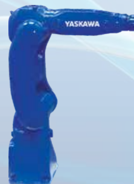
ROBOT MODEL GP 8 Payload: 8 Kgs. Horizontal reach: 727 mm
