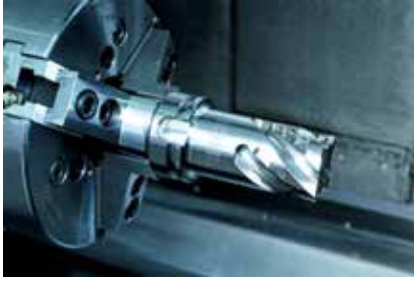
Finished Igel milling cutter with HSK shaft
