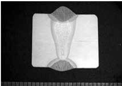
Fig.4b. macro section showing MAG root and cap beads & central hybrid weld bead
