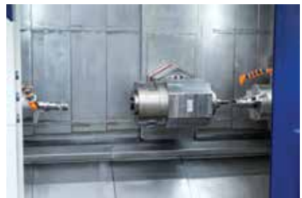
More space for the machining of complex workpieces, distance between the spindles: 1400 mm
