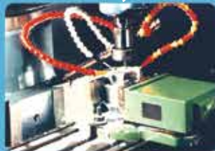
Flexible Coolant Pipes
